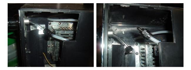
3.) Then, while pulling the tower lever down (as if opening to pour beer), pull the hose out from the back side as pictured below.
